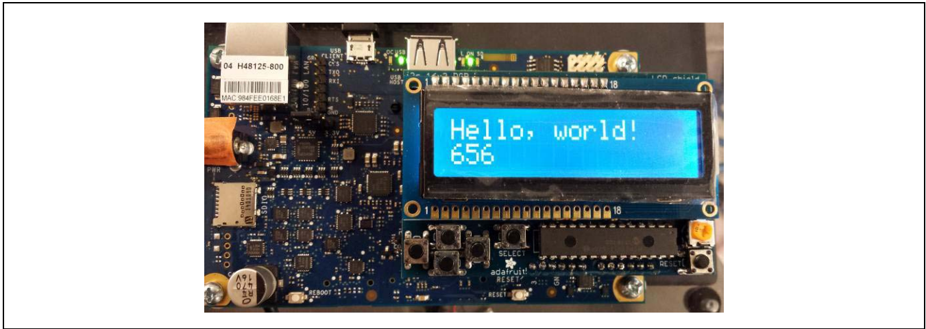
Figure 50 Adafruit* I 2 C RGB LCD shield kit with 16 × 2 display on Intel® Galileo second generation
