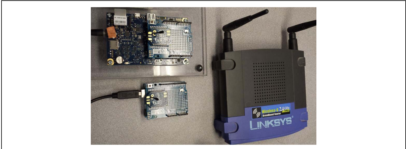
Figure 156 XBee® Wi-Fi module shield, shown with an Arduino® Uno board and an Intel® Galileo second generation board
